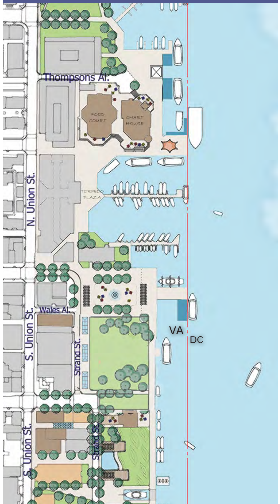
Figure 22: Illustrative Plan showing a Marina Arrangement Extending only to the Pierhead Line
