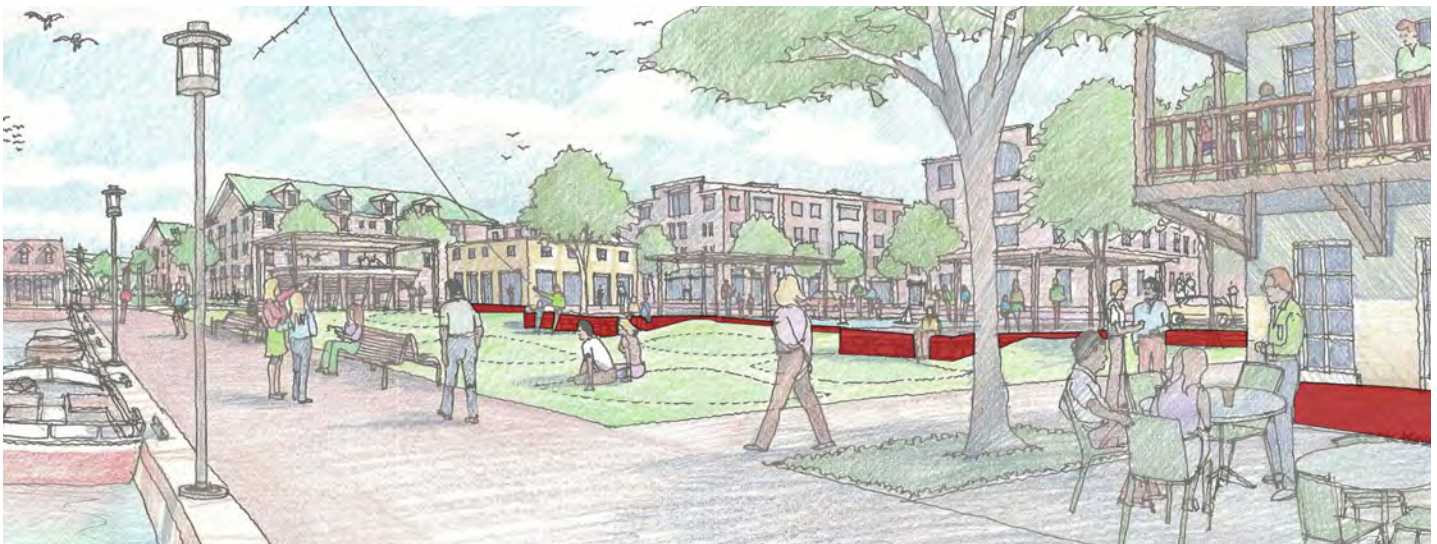
Artists Perspective showing how proposed flood mitigation can be integrated into the building and park design. Here, flood control is highlighted - along building facade at a repurposed Beachcomber, through grading, and integrated into a series of pier-like structures in an Expanded Point Lumley Park.
